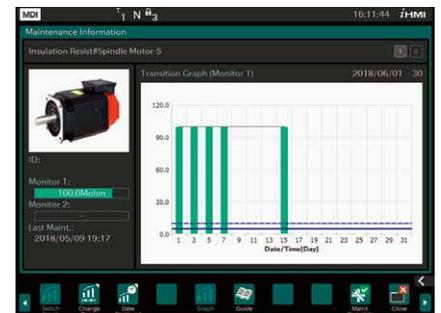
Leakage Detection Function
